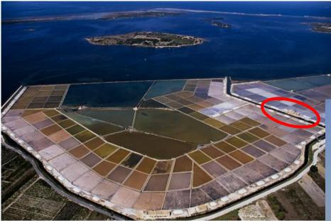
Direct access to both saturated brine and seawater from open channels
